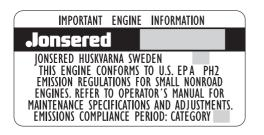
The Emissions Compliance Period referred to on the Emissions Compliance label indicates the number of operating hours for which the engine has been shown to meet Federal emission requirements.
